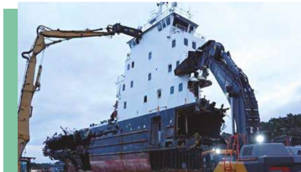
Nordic Circles in Norway transforms ships and oil rigs into environmentally friendly building products. The start-up company acquired steel from this former ferry to build urban quays that also function as “fish hotels” bringing marine life back to city port. To upcycle the steel, pieces are cut out from the car deck and transported to regional steel production partners around Bergen. (Source: Nordic Circle, October 2021) https://www.nordiccircles.com/news/nordiccirclesattedx-eps2g-h763c-ft3yh
